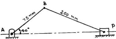
For the crank position indicated, find (i) the angular velocity of the connecting rod BP. (ii) Velocity of piston P. (AU, Dec"11, Jun"10)
