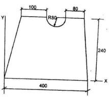
**32.** Determine the principal moments of inertia and find location of principal axes of surface shown in fig.
