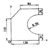
**31.** Find the moment of inertia of a section shown in Fig below about the centroidal Axes.(Dimensions in mm) (AU JUN"09)
