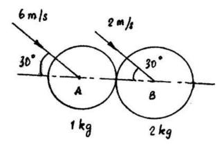
If the coefficient of restitution is 0.5, find the velocity and the direction the two balls after impact. Also calculate the loss in kinetic energy due to impact and the percentage of loss. (AU, Dec"10, Jun"12)
