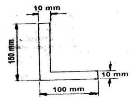
**30.** Locate the centroid of the area shown in figure below. The dimensions are in mm. (AU JUN"10, DEC 11)
