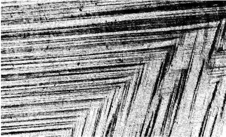
Figure 5.3 Slip lines in copper.
