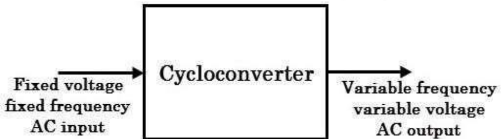
Figure 5.7.1 Block diagram of cyclo converter
