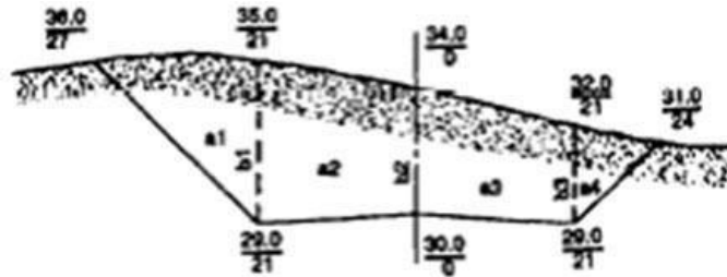
Fig. 24.6. Cross Section Cut Showing Distances and Elevations
