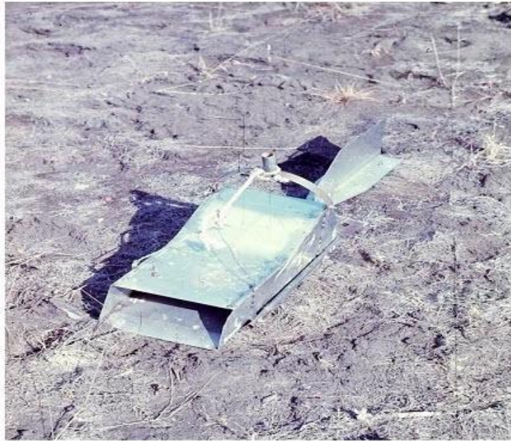
Fig. 20.1. A Commonly Used Type of Bed-load Sampler.
