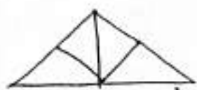
King Post truss. (upto 6m span)
