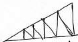
North light truss. (8m to 10m)
