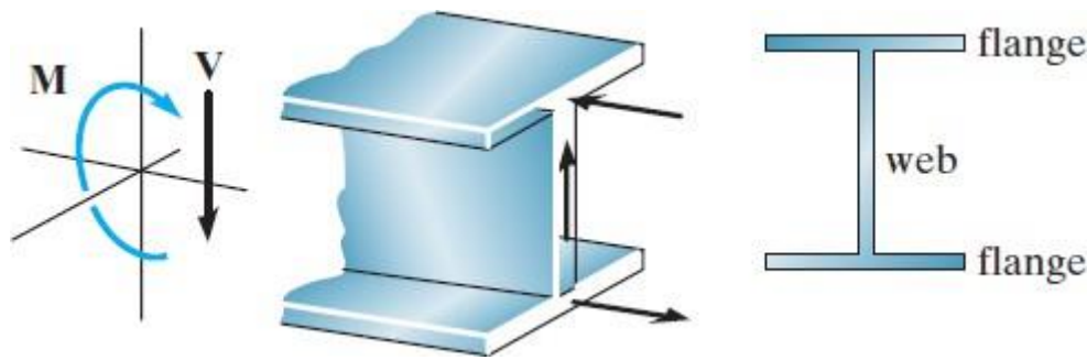
Figure 5.2 Cross section of a beam
