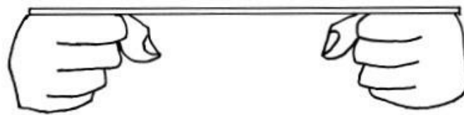
(a) Ruler simply supported on two fists
