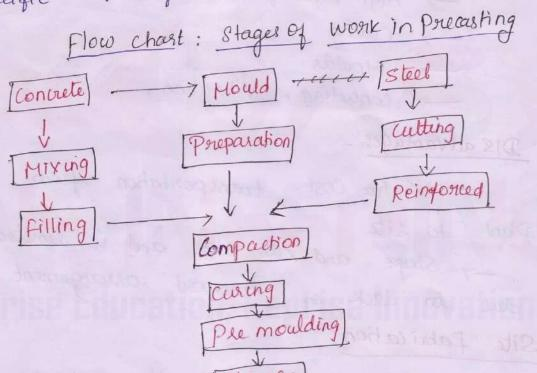
Methods for Manufacture of precast concrete
